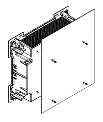
The section that extends outside the frame of the board is to protect the incoming mains cables. The plate can be reoriented to suit either direction.
